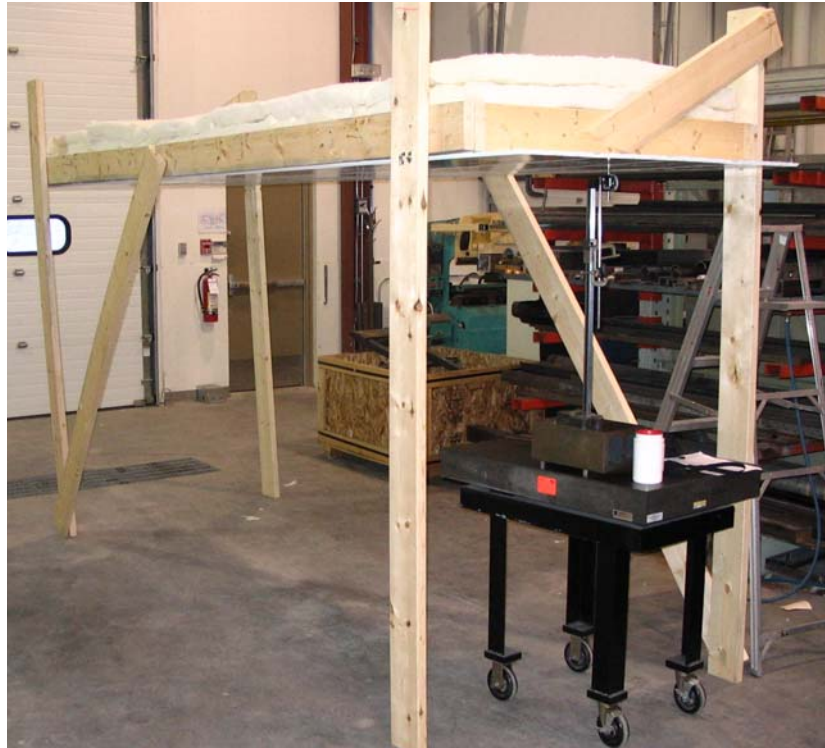
Figure 2 – Panels Loaded with Insulation
